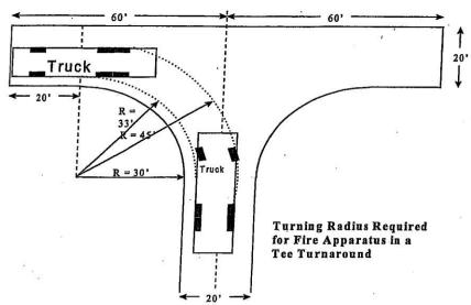
The 20 ft access width is a minimum for use only with an exclusive fire department emergency access way. For roadways or public streets, these access widths must be increased. The end length of 60 ft may remain the same, however. Variations of this hammerhead are shown below:
